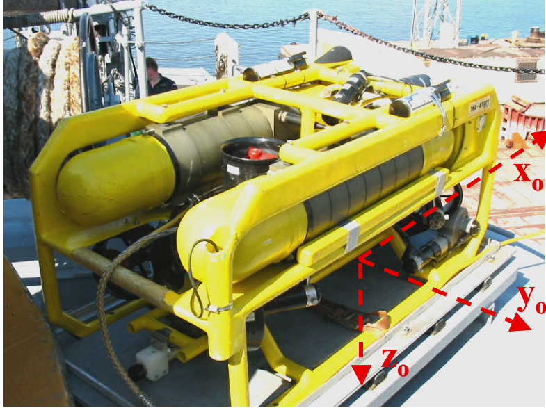
Fig. 1. Remotely operated vehicle Ukwial on board of countermine warship
