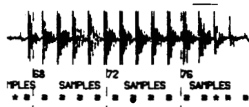
Fig. 17. Example indicating possibility of extra acoustic segments for a given phonetic segment. The waveform plot is similar to the one described in Fig. 16. The vowel /æ/ has significantly different parameters for the last 50 ms or so (from time unit 75 onwards) making it a candidate for an extra acoustic boundary.
