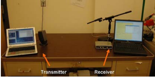
Fig. 1. OFDM testing in air: testbed (left) and typical channel impulse response (right)
