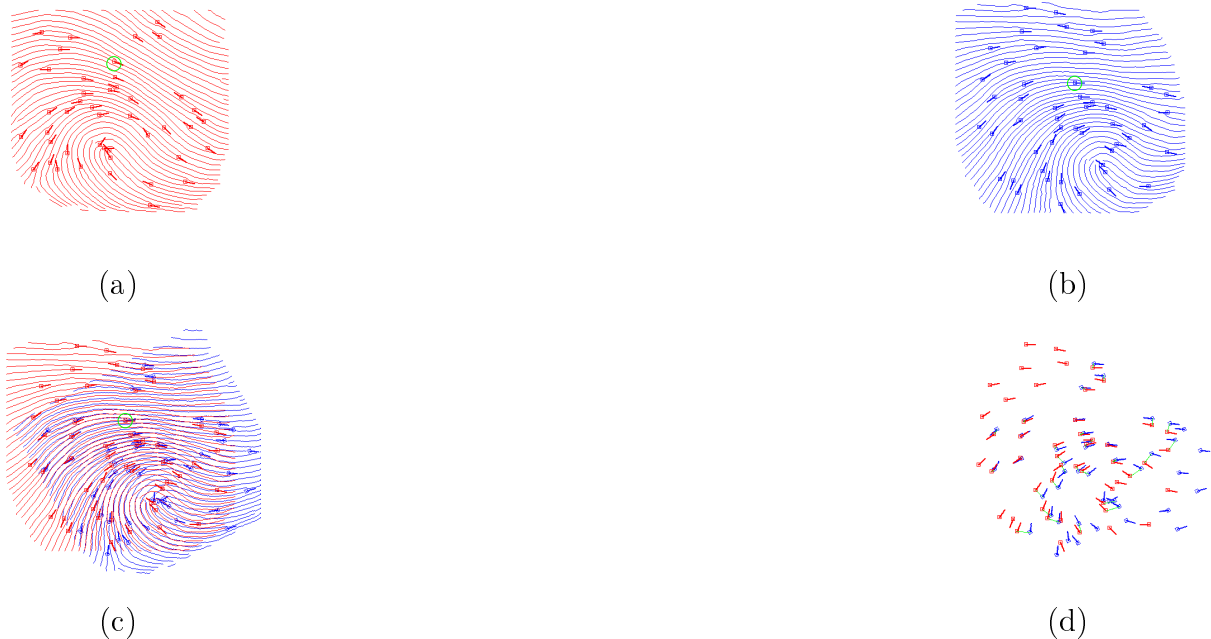
Figure 12: Results of applying the matching algorithm to an input minutia set and a template; (a) input minutia set; (b) template minutia set; (c) alignment result based on the minutiae marked with green circles; (d) matching result where template minutiae and their correspondences are connected by green lines.
