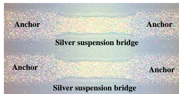
Fig. 6. Silver suspension bridges, fabricated using basic MaSPrint processing [90].
