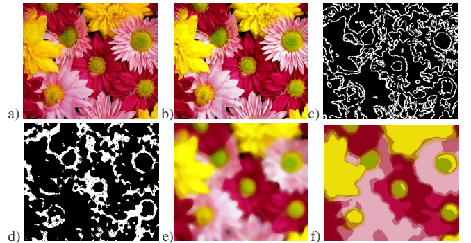
Fig. 4: a) Original image, b) color-constancy processed image, c) edges and transition regions (white), d) textured regions (white), e) smoothed image, and f) color segmented image.
