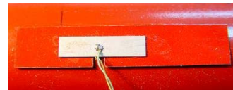
Fig. 5. Piezoelectric sensor for collecting strains
