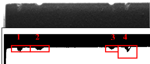
Fig. 8. Exemplary results for tile with damaged edge.
