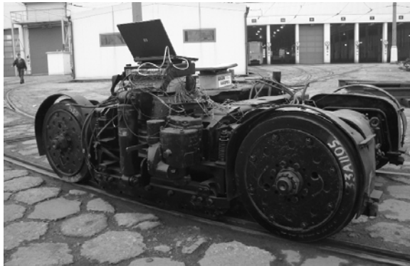
Fig. 3. Measuring test bogie equipped with measurement set
