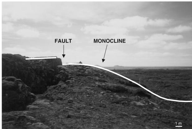
Fig. 3. Typical features along fracture zones in the Vogar fissure swarm. In this example, a surface monocline is breached by a fault along its upper hinge line. The fault displays both vertical and opening displacements and the fault scarp is vertical.
