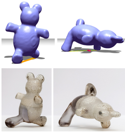
Figure 13: (Top) This Teddy bear has been edited and optimized to stand in two different positions. (Bottom) The printed object stands in both configurations. We intentionally printed in transparent material to reveal the uneven distribution of weight inside.
