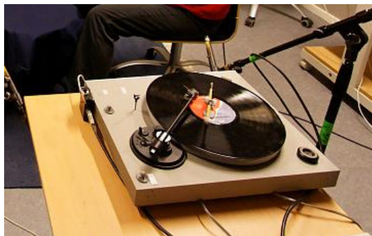
Figure 2: The turntable in action. In addition to the reflecting marker mounted on the record, two markers fixed at a set distance on the side of the turntable serve as a distance reference.
