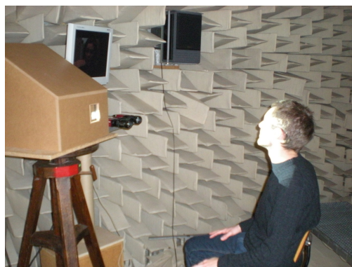
Figure 2: Recording setup: one speaker sits in front of the 3D scanner in the anechoic room while watching a video for instructions on the screen.
