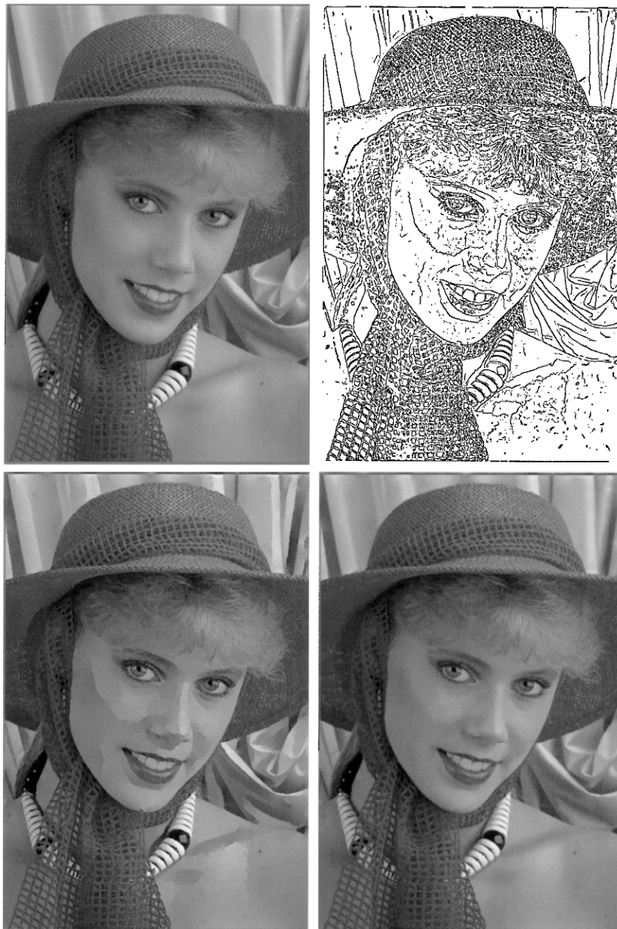
Figure 15. Top left: Original image. Top right: Detected edges. Bottom left: Reconstructed luminance function. Bottom right: Reblurred result. Reblurring is critical to capturing the smooth shading of the skin. Edge density is 18%, and RMS error for this reconstruction is 5.0 grey levels, including a 0.1 grey-level DC component, and an estimated 1.7 grey levels due to noise removal.
