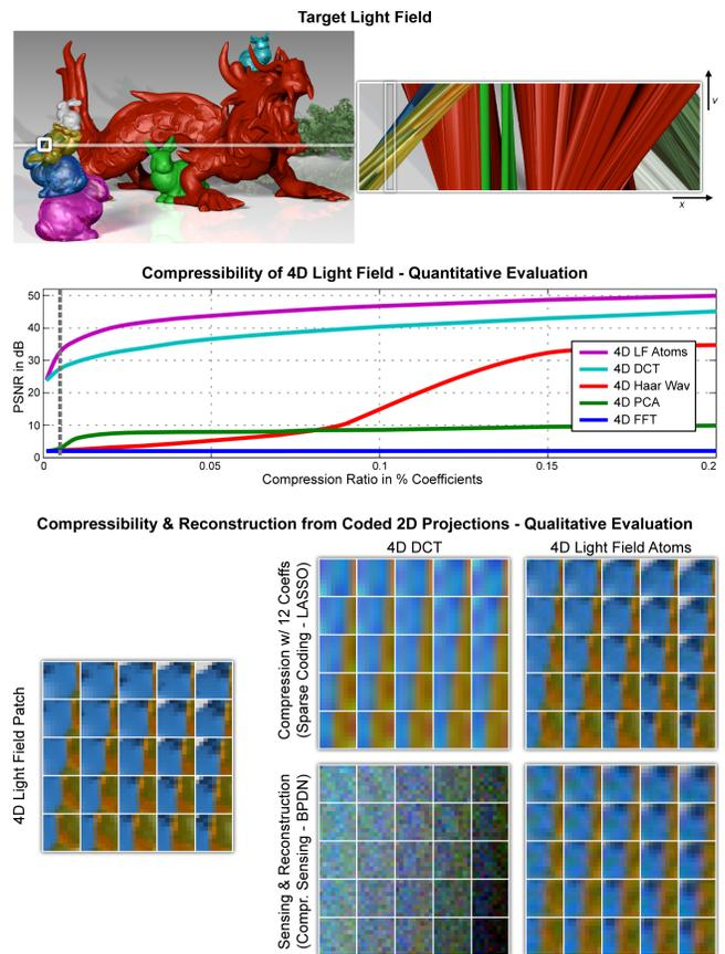
**Figure 2:** Compressibility of a 4D light field in various high-dimensional bases. As compared to popular basis representations, the proposed light field atoms provide better compression quality for natural light fields (plots, second row). Edges and junctions are faithfully captured (third row); for the purpose of 4D light field reconstruction from a single coded 2D projection, the proposed dictionaries combined with sparse coding techniques perform best in this experiment (bottom row).
