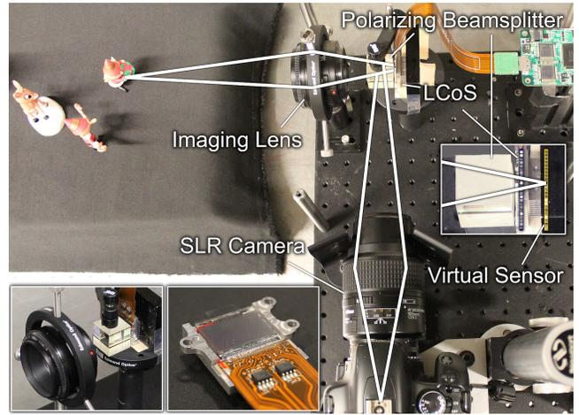
**Figure 9:** Prototype light field camera. We implement an optical relay system that emulates a spatial light modulator (SLM) being mounted at a slight offset in front of the sensor (right inset). We employ a reflective LCoS as the SLM (lower left insets).
