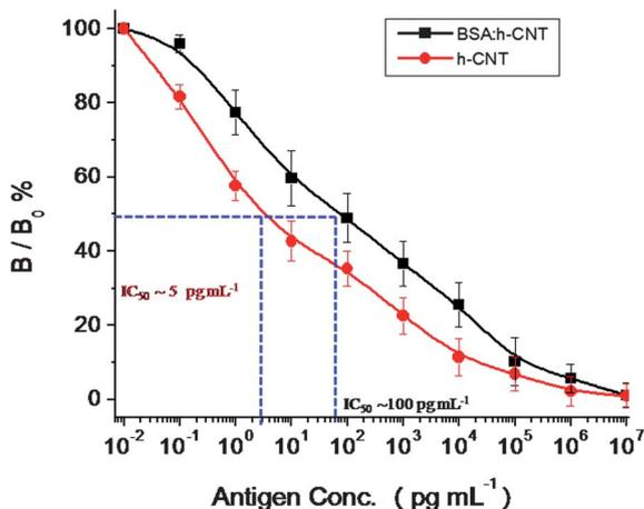
**Fig. 7** Competitive electrochemical inhibition assay ( $n = 3$ ) of diuron using (●) direct hapten coated CNTs functionalized SPE and (■) BSA-DCPU conjugate coated CNTs functionalized SPE. The concentration of diuron was selected between  $10^{-2}$  to  $10^7 \text{ pg mL}^{-1}$ .
