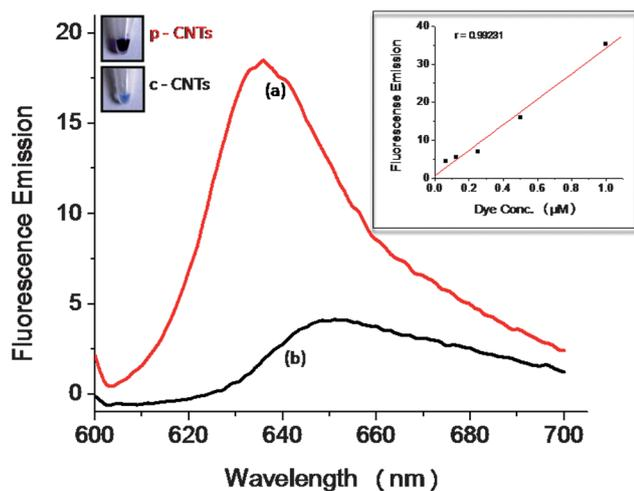
**Fig. 2** Fluorescence spectra of (a) carboxylated and (b) pristine CNTs respectively. A standard curve of THA dye was prepared by taking different concentration (0.125–1  $\mu\text{M}$ ) of the dye. Inset shows the change in color from deep blue to purple for carboxylated CNTs depicting the extent of carboxylation on CNTs in presence of dye.
