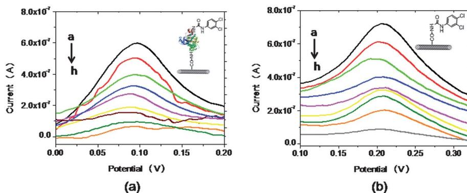
**Fig. 6** Response curves (left) DCPU-conjugate coated c-CNTs modified SPE and (right) h-CNTs on SPE at different concentrations of diuron samples (a–i) 0 to  $10^6$   $\text{pg mL}^{-1}$  free diuron respectively. The signal was measured as oxidation of 1-naphthol after 10 min incubation in Tris pH 8,  $\text{MgCl}_2$ , differential pulse voltammetry technique at amplitude 50 mV, pulse width 0.2 s, pulse period 0.5 s.
