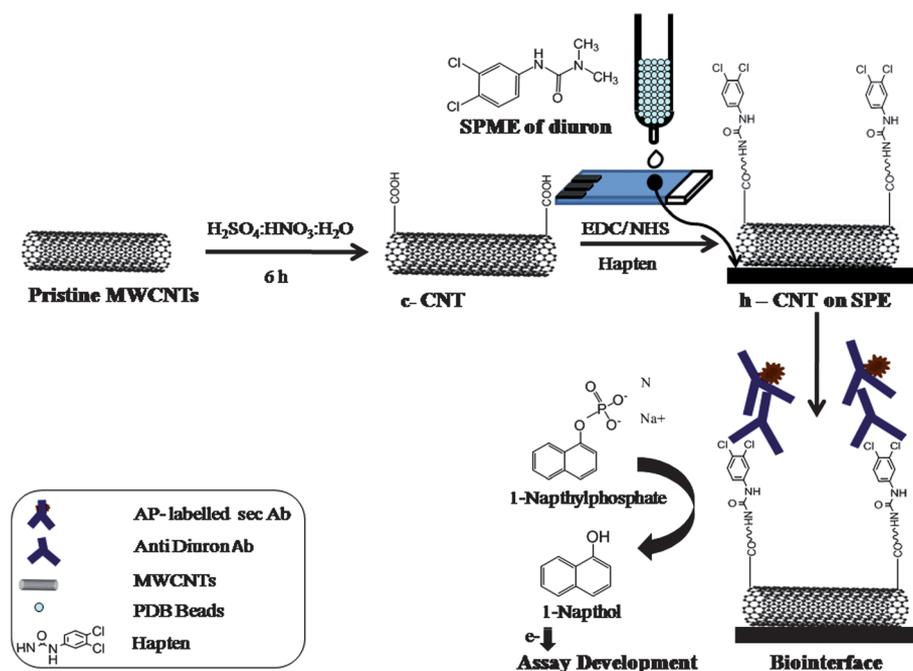
**Scheme 1** Schematic representation of SPME micro-cartridge column coupled with an EIA using haptens on CNTs for the monitoring of phenyl urea herbicide. The pristine CNTs were carboxylated by acid treatment followed by haptensation using carbodiimide chemistry for assay development.
