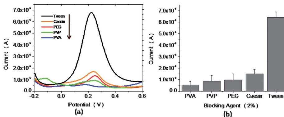
**Fig. 5** Blocking efficiency of various blocking agents in terms of (a) DPV Scans and (b) the corresponding current signal response observed in the electrochemical assay ( $n = 3$ ).
