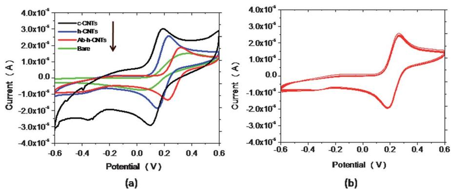
**Fig. 4** (a) CV scans of CNTs functionalized SPE (c-CNTs, h-CNTs, Ab-h-CNTs and bare electrodes respectively) and (b) presents the no. of scan cycles (25 cycles) of h-CNTs on SPE. The scans were obtained in 2.5 mM ferrocyanide prepared in PBS (pH 7.4) at a scan rate 50 mV s<sup>-1</sup>.
