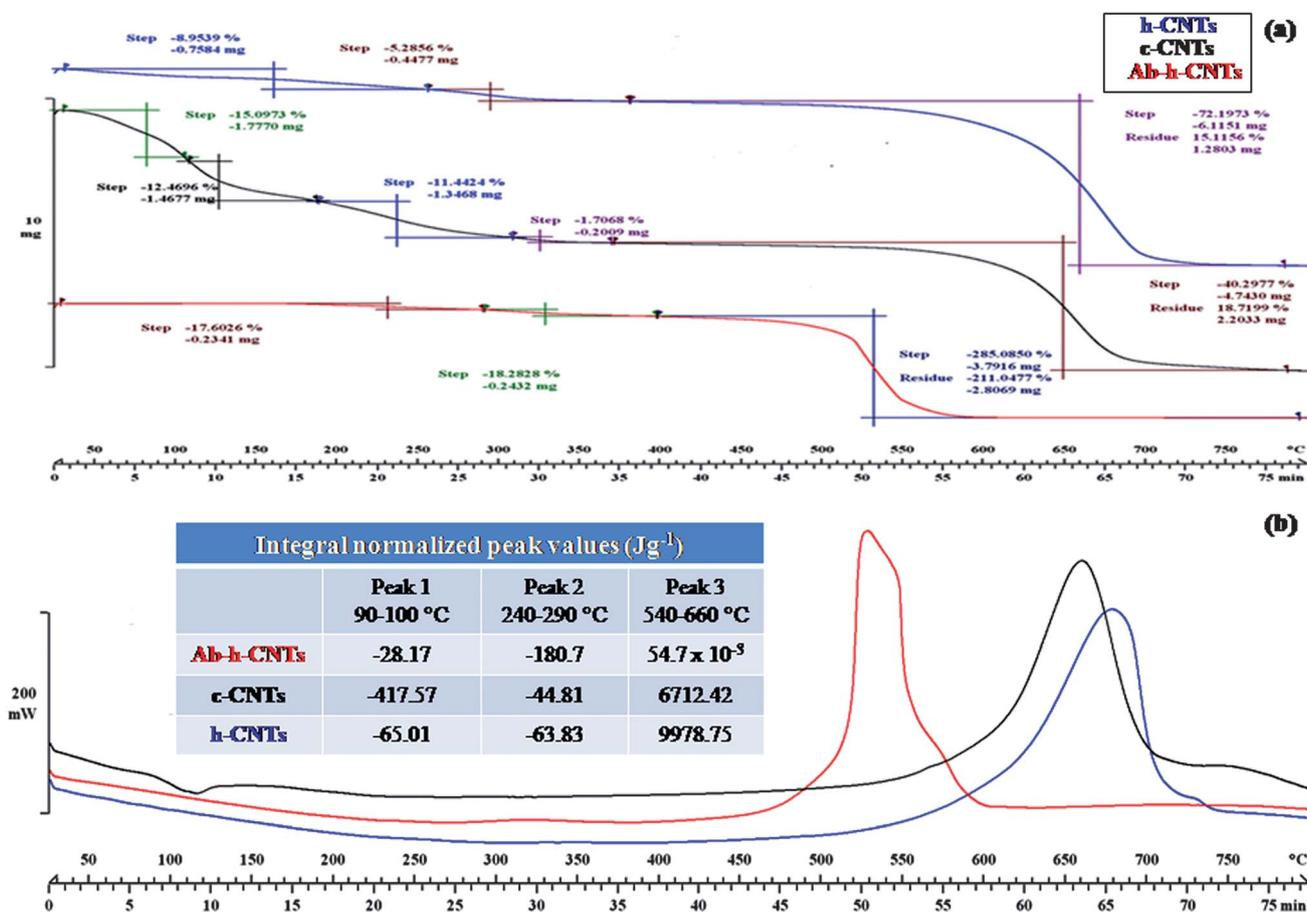
**Fig. 3** (a) Percentage weight loss vs. decomposition temperature by TGA analysis for c-CNTs, h-CNTs and Ab-h-CNTs respectively and (b) shows the DSC analysis of c-CNTs, h-CNTs and Ab-h-CNTs respectively. Inset (table) shows the normalized integrated values calculated from the respective peak area. Heat rate was selected at 10  $^{\circ}\text{C min}^{-1}$ .
