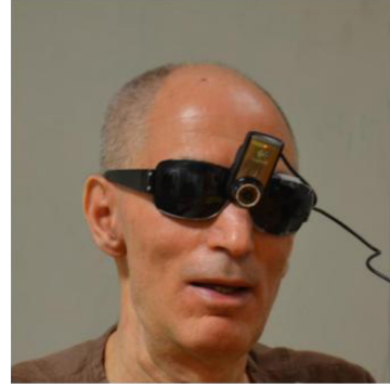
Fig. 11. Example setup of clothing pattern recognition prototype to capture images by a web camera with auto focus on sunglasses.
