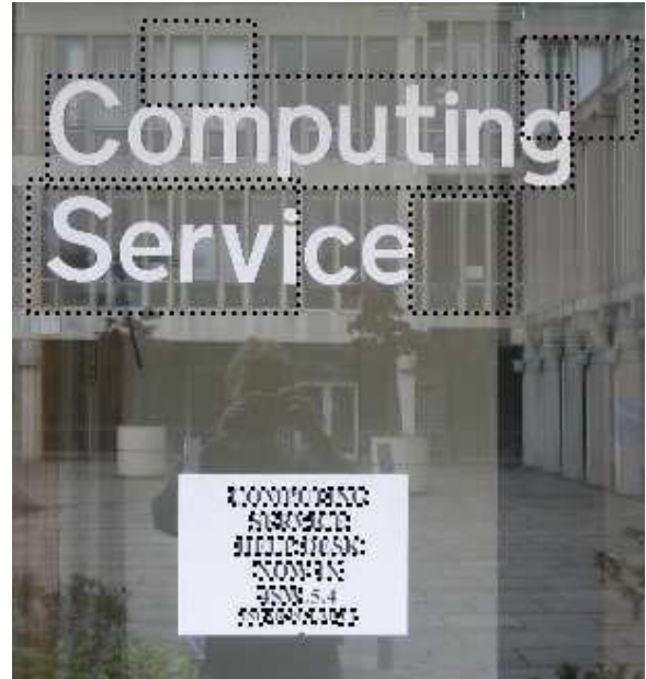
Figure 4. An image uploaded to the Alex Chen algorithm, installed as a web service. The located rectangles are shown in black dotted lines.
