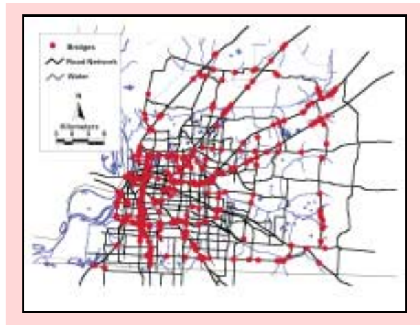
■ Figure 2. Shelby County Tennessee Highway System Model (7,807 Links and 15,604 Nodes)
