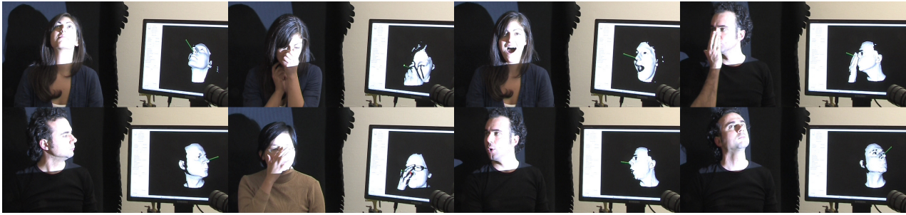
Figure 10. Example frames from our real-time head pose estimation system, showing how the regression works even in the presence of facial expressions and partial occlusions.
