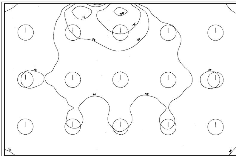
**Figure 8** Contour plot of working plane illuminance (lux) in example room lit by passive pipes and vertical windows
