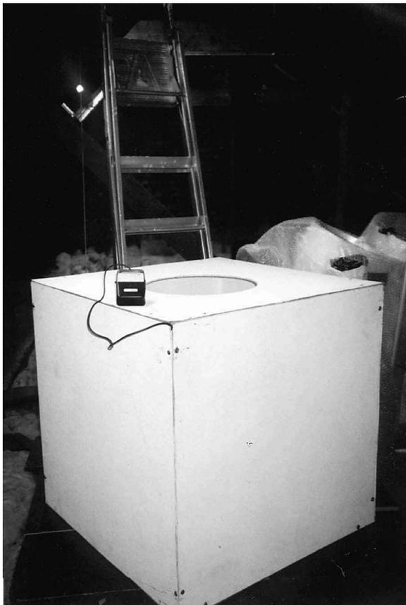
**Figure 2** Photometric integrator for luminous flux measurement
