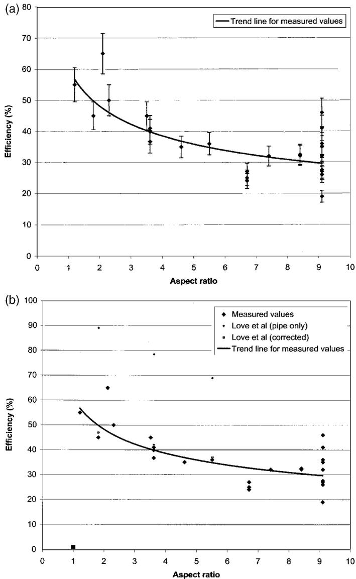
**Figure 5** (a) Graph of pipe efficiency against aspect ratio. (b) Graph of pipe efficiency against aspect ratio
