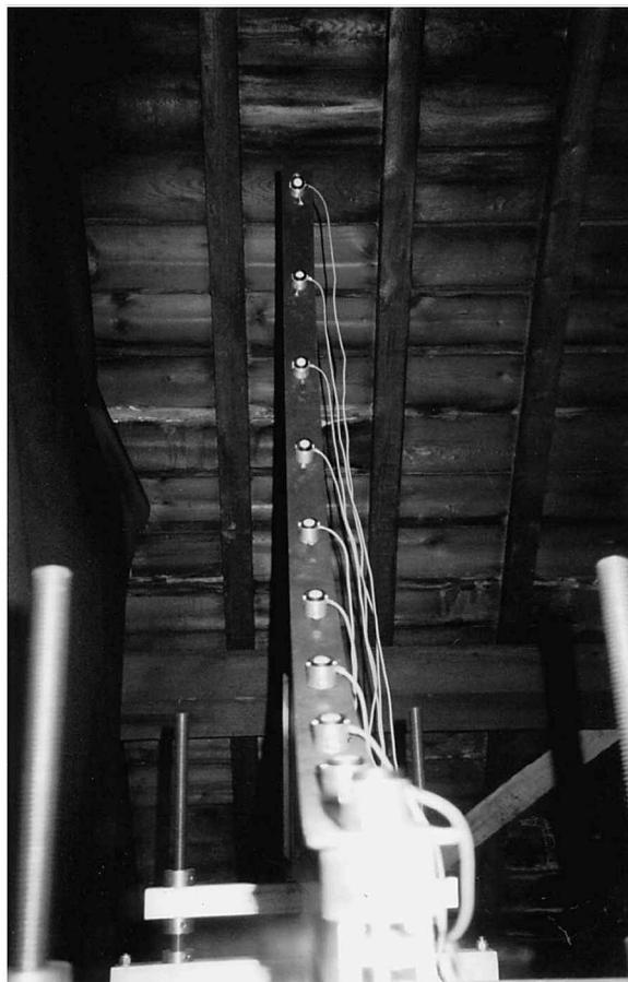
**Figure 1** Apparatus to measure luminous intensity distribution from pipe emitter
