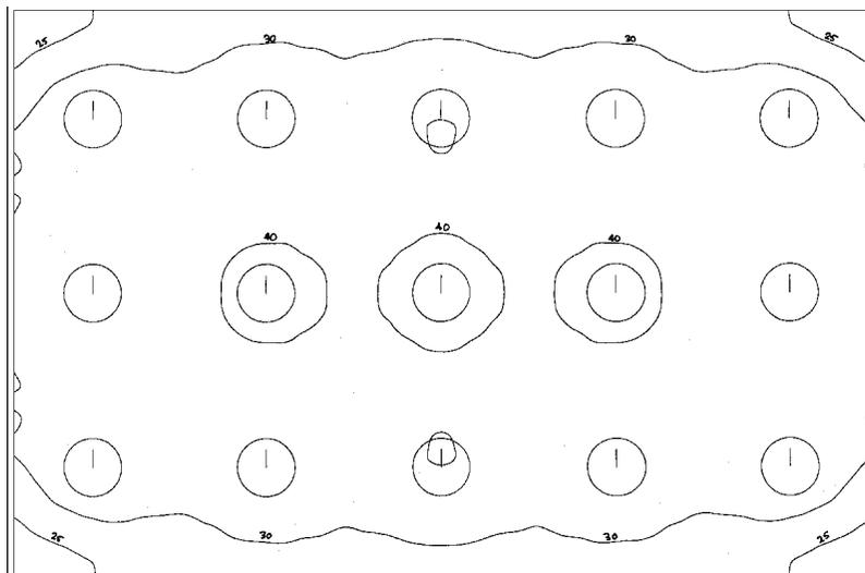
**Figure 7** Contour plot of working plane illuminance (lux) in example room lit by passive pipes
