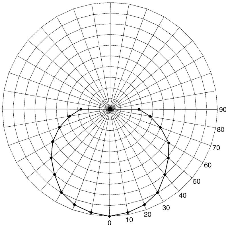
**Figure 4** Polar curve of average luminous intensity distribution for overcast sky (Nadir intensity = 295 cd/10001 m)
