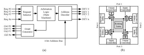
Fig. 4. Block diagram of the: (a) bus control unit used in the bus; and (b) on-chip router in the NoC implementation.
