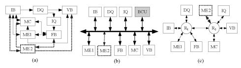
Fig. 5. Implementation of MPEG-2 encoder with 2 MEs using: (a) P2P; (b) bus and (c) NoC communication architectures.
