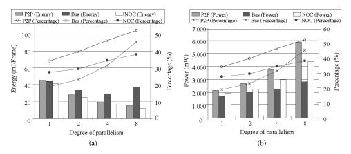
Fig. 9. (a) Energy consumption; and (b) power consumption (mW@ 100MHz) as a function of the degree of parallelism for P2P, bus, and NoC implementations.
