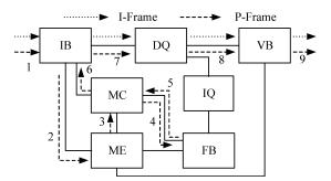
Fig. 7. Critical paths for I-Frame and P-Frame encodings are shown with dotted and dashed lines, respectively.
