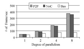
Fig. 8. Throughput comparison of various MPEG-2 encoder implementations.
