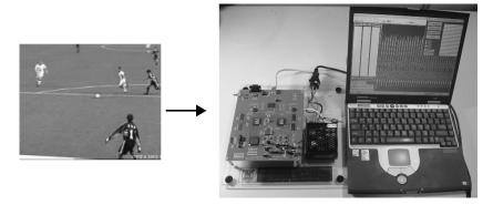
Fig. 3. The FPGA prototype running the MPEG-2 encoder as demonstrated at the UBooth, Design Automation Conference in July 2006.
