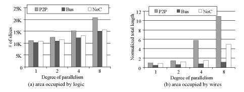
Fig. 6. Area comparisons of the MPEG-2 encoder implemented using P2P, bus, and NoC architectures for increasing levels of parallelism.
