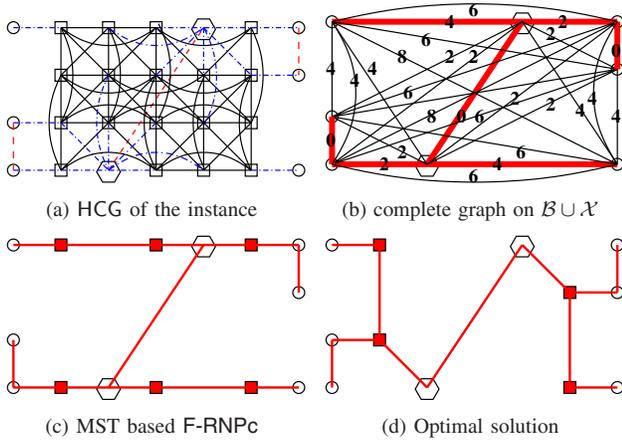
Fig. 2. (a) The HCG for two BSs (hexagons), six SNs (circles), and 18 candidate locations for RNs (squares). (b) The edge-weighted complete graph on  $\mathcal{B} \cup \mathcal{X}$  where the edge weight is the shortest path length in the HCG, and an MST (thick edges). (c) The corresponding F-RNpc, which uses six RNs. (d) The optimal solution, which uses four RNs.
