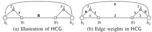
Fig. 1. (a) shows  $\text{HCG}(r, R, \{b_1, b_2\}, \{x_1, x_2\}, \{y_1, y_2\})$ , where  $d(x_1, b_1) = d(x_1, y_1) = d(x_2, b_2) = d(x_2, y_2) = r$ ,  $d(y_1, y_2) = R$ . (b) shows the edge weights, where an edge incident with no relay node has a weight of 0, an edge incident with exactly one relay node has a weight of 1, and an edge incident with two relay nodes has a weight of 2.
