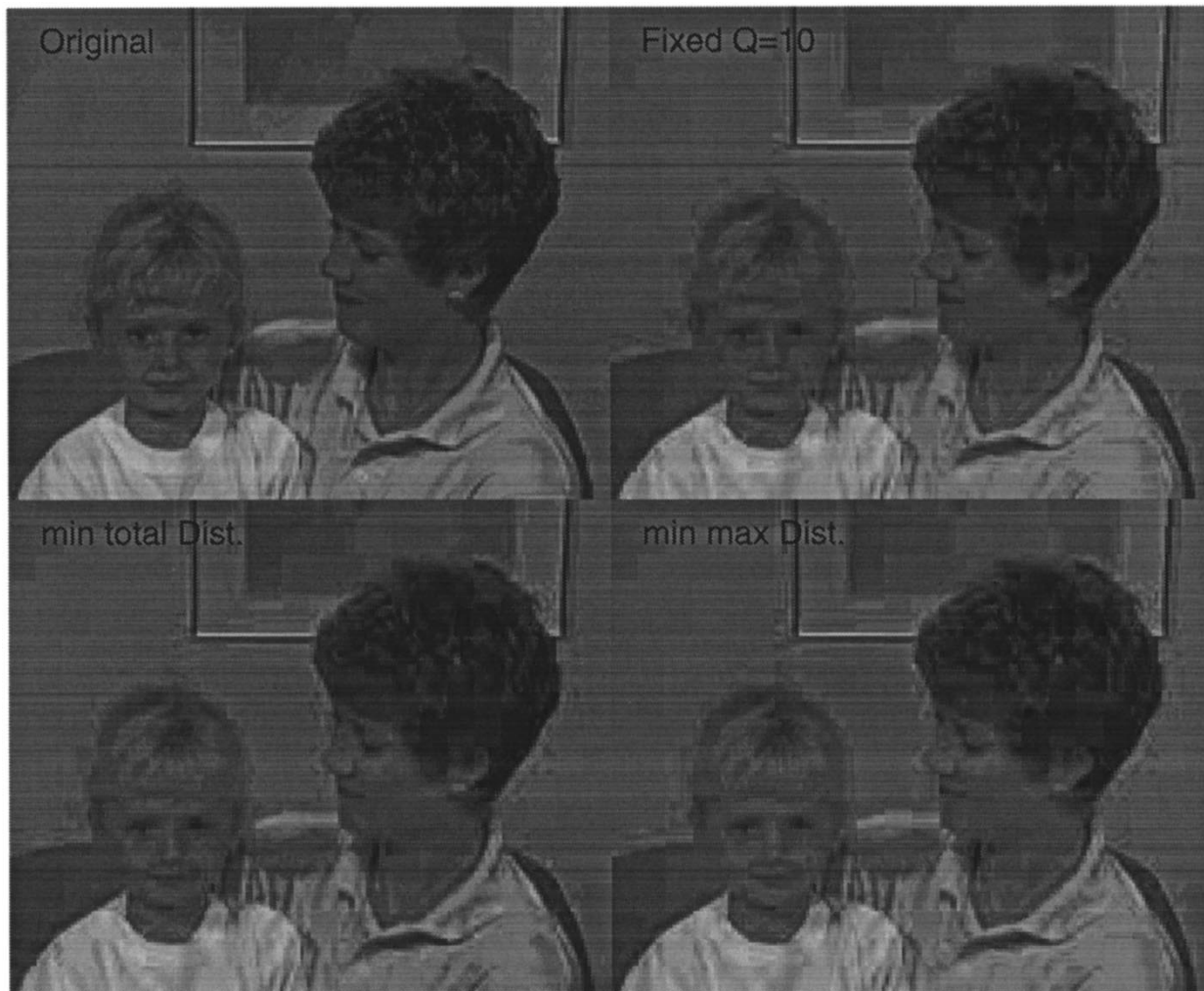
Fig. 4. Comparison between MINMAX, MINAVE, and fixed quantizer approaches with the same compression ratio.
