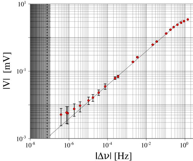
Fig. 4. Measured voltage  $|V|$  as a function of the Doppler shift  $\Delta\nu$ . The dotted line and the gray region represent the photon shot noise. The continuous line is the fit of the linear part of the response.
