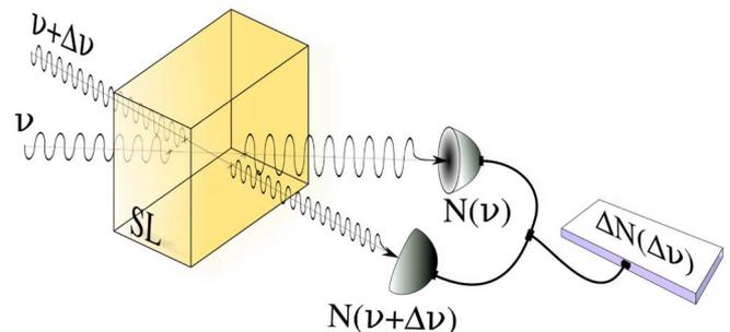
Fig. 1. Two-beam interaction in a slow-light (SL) medium. Two nondegenerate light beams of the same intensity and with a slightly different frequencies,  $\nu$  and  $\nu + \Delta\nu$ , respectively, interact in the SL medium. The difference  $\Delta N$  between the output intensities, which is measured through a balanced detection, strongly depends on the Doppler shift  $\Delta\nu$ .
