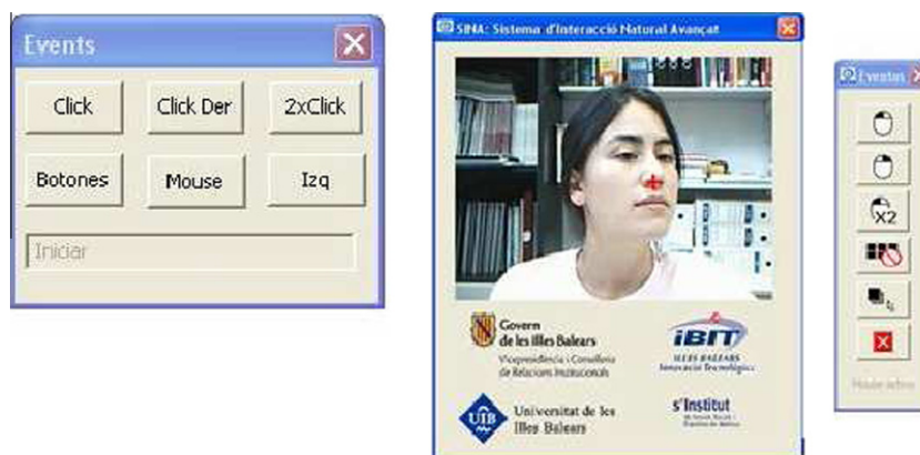
Fig. 5. Interface (a) event toolbar with text and (b) event toolbar with images.
