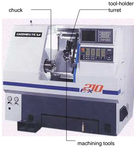
Fig. 2. A turning center and its tool-holder turret.
