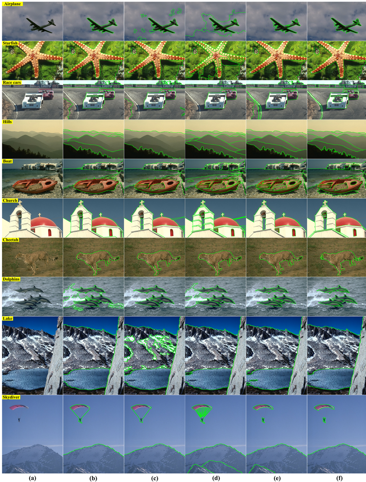
Fig. 1 Berkeley segmentation benchmark: 1 (a) original images, and (b) to (f) region boundaries of multiple manually generated segmentations overlaid on the images.
