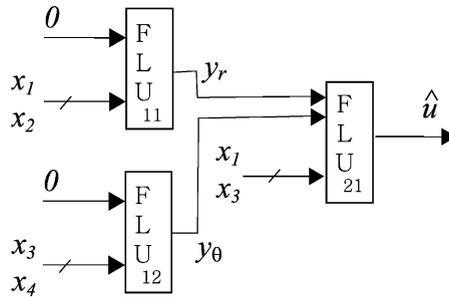
Fig. 6. A controller for ball and beam system.
