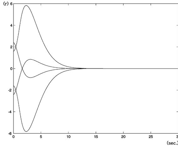
Fig. 5. Output  $r(t)$  of the closed loop ball and beam system from four initial conditions when the input–output linearization algorithm of Hauser et al. is used.
