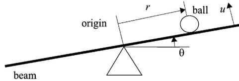
Fig. 4. The ball and beam system.
