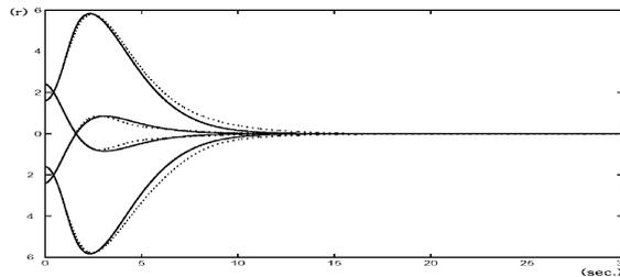
(b)  $r(t)$  of the closed loop ball and beam system (solid : results with the input-output linearization algorithm, dotted : results with the proposed controller)
