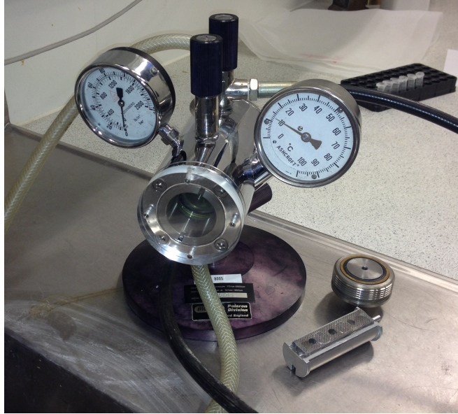
Figure 8: Critical Point Drying system, with a pressure and temperature measuring system on the left and right side, and a small chamber in the middle where the small wire cage is kept during the drying procedure.
