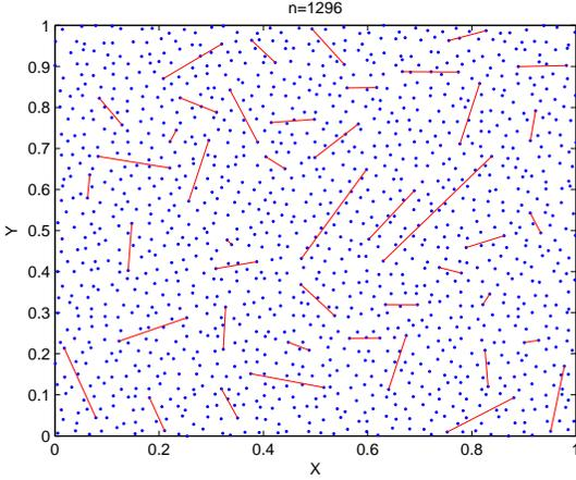
Figure 3: A possible assignment of source-destination pairs for simultaneous end-to-end communication in a 1296-node network, where each assigned source-destination pair is represented by a line segment connecting the source and the destination.
