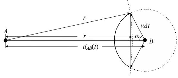
Figure 1: The illustration of the approximation (3) when node B is outside of the transmission range of node A at time  $t$ .
