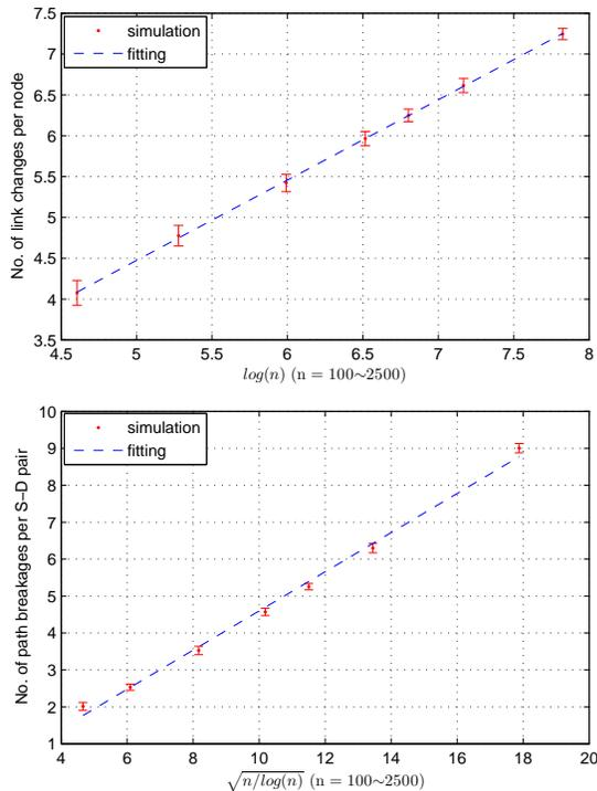
Figure 5: Upper: the number of link changes per node in networks with different sizes ( $n = 100 \sim 2500$ ); The x-axis uses a  $\log n$  scale. Bottom: the numbers of path breakages per source-destination pair in a time slot networks with different sizes ( $n = 100 \sim 2500$ ); The x-axis uses a  $\sqrt{n/\log n}$  scale. The error bars show the 95% confidence interval.
