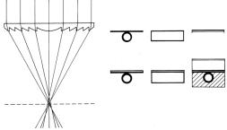
Figure 1: The geometry of the linear Fresnel lens, with indication of the concentrating solar radiation (left) and alternative absorbers of Thermal (T), PV and PVT type (right).
