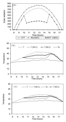
Figure 4: Solar radiation and temperature results for system operation at 20°C and 50°C from 10:30 to 14:30.
