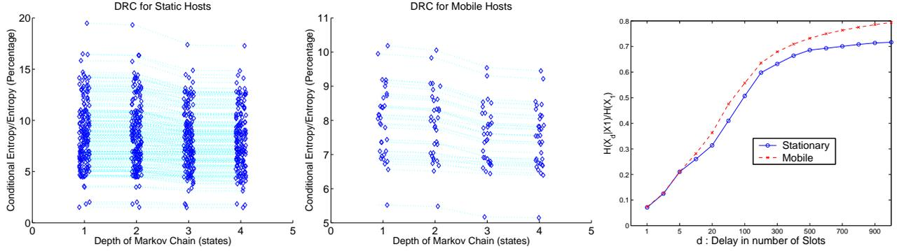
**Figure 5: Reduction in normalized conditional entropy as a function of past  $n$  slots: Stationary Hosts (Left) and Mobile Hosts (Middle); and Normalized Conditional Entropy as function of lag  $d$  (Right).**
