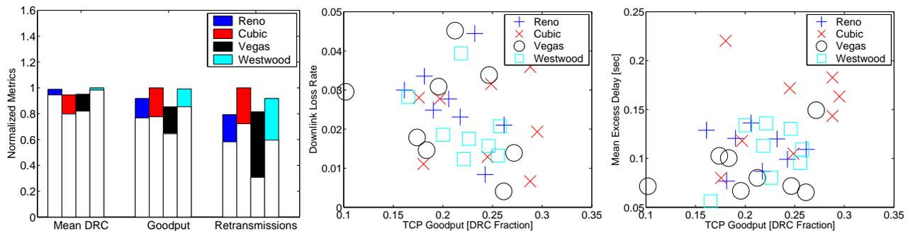
**Figure 10:** For  $EX_{TBED}$ : (Left) TCP Goodput, Mean DRC and the average fraction of packets that were retransmissions (height of the bars normalized w.r.t the maximum in the group). The colored portions show the magnitude of the standard deviations. (Middle) End-to-end loss rate, and (Right) Mean delay.
