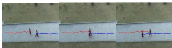
Figure 7 Tracking results of multi-people by our algorithm with occlusions (frame 72, 103, 134, 165, 196, 227)
