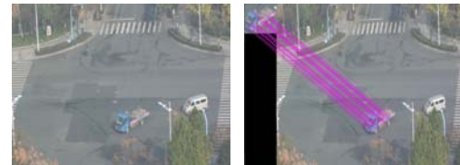
Figure 2 Matching of SIFT features between target and the candidate target
