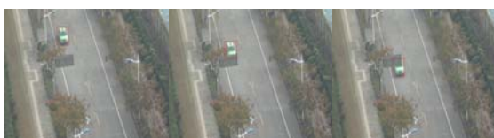
Figure 8 Tracking results of multi-vehicles by the traditional Camshift with occlusions (frame 65, 76, 87, 98, 109, 120)
