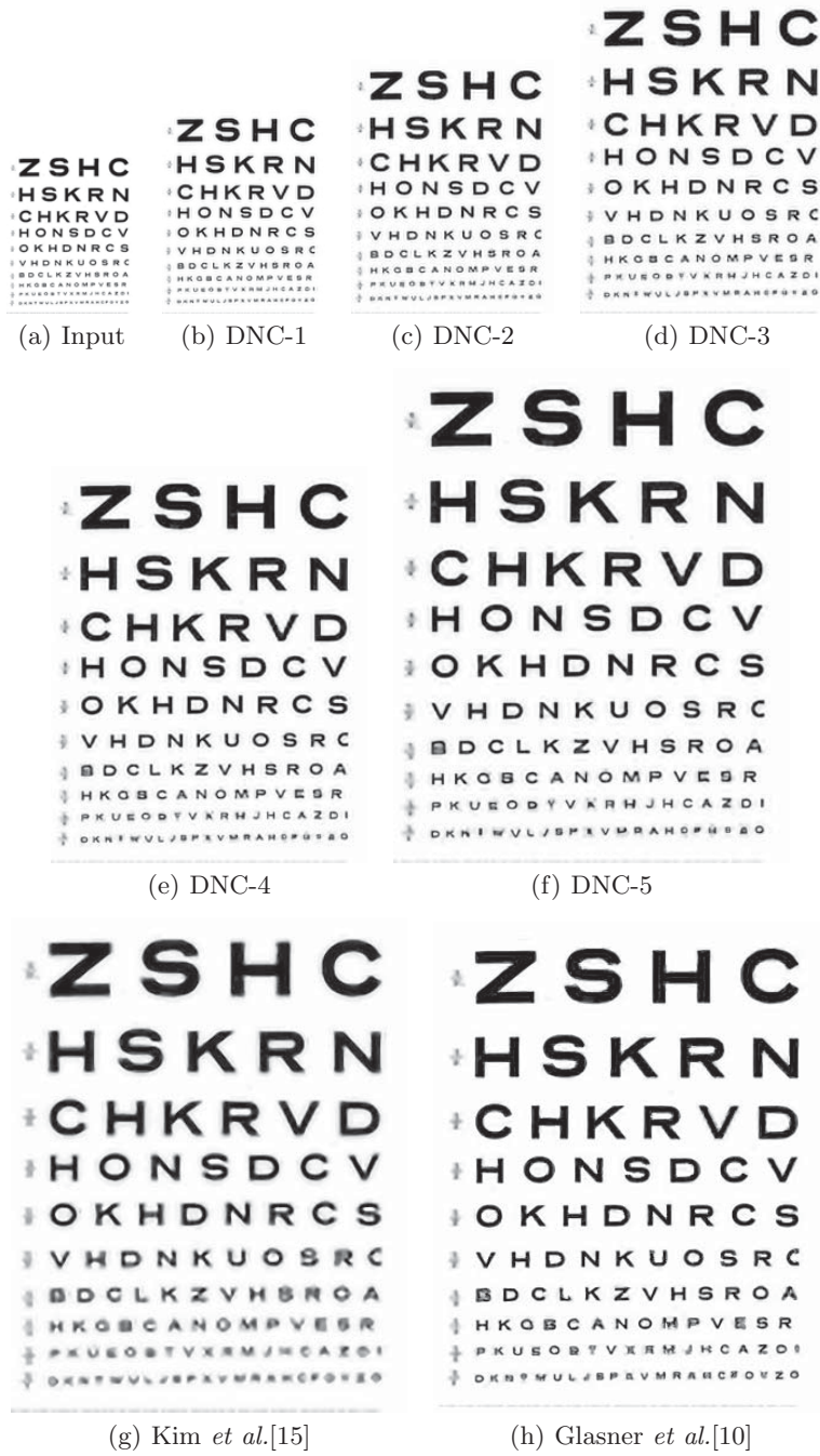
Fig. 2. An example of gradual SR by 3\times . The proposed network cascade magnifies the input LR image layer by layer in (b)-(f). Please zoom PDF with 324 \times 405 pixels.
