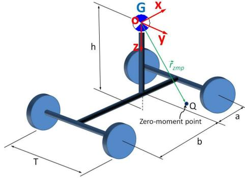
Fig. 2: Rigid vehicle model
