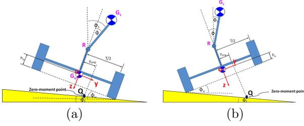
Fig. 5: Vehicle roll model on terrain. (a)  $\phi_u \geq \phi_t$  (b)  $\phi_u < \phi_t$
