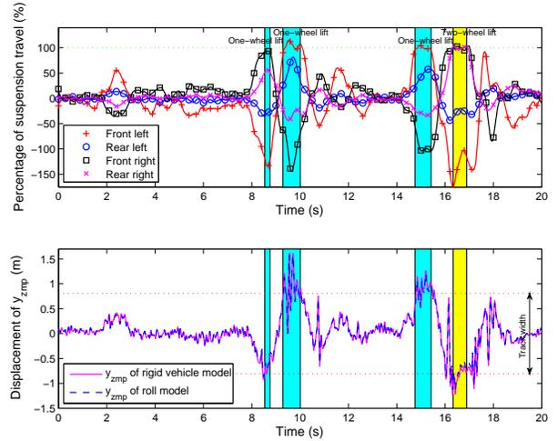
Fig. 8: Percentage of suspension travel and displacements of  $y_{zmp}$  of vehicle during double-lane change on flat road at 10 m/s, causing wheel liftoff.
