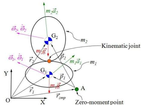
Fig. 1: Two-link kinematic chain
