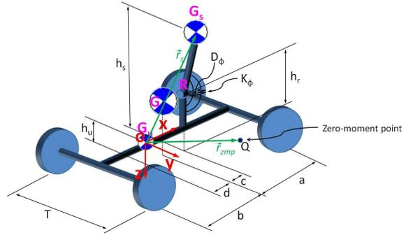
Fig. 4: Vehicle roll model
