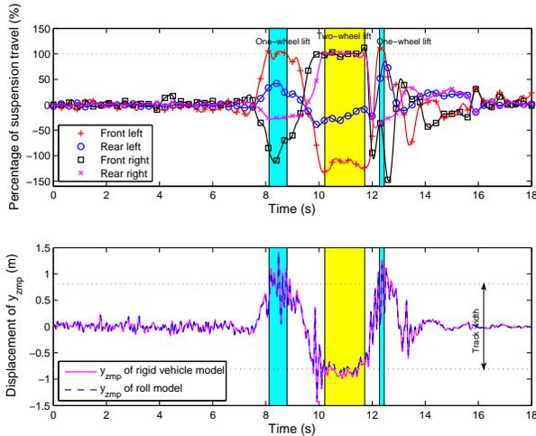
Fig. 7: Percentage of suspension travel and displacements of  $y_{zmp}$  of vehicle during Toyota’s J-turn on flat road at 10 m/s, causing wheel liftoff.
