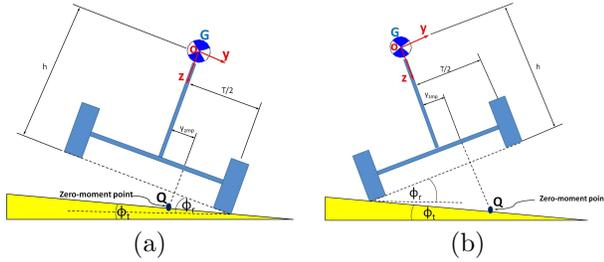
Fig. 3: Rigid vehicle model on terrain. (a)  $\phi_r \geq \phi_t$
