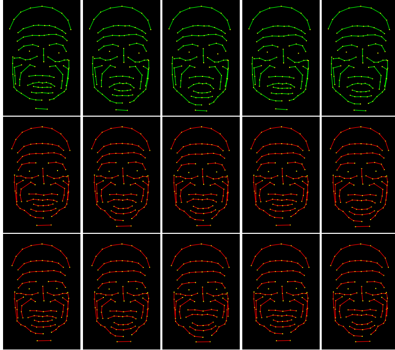
Fig. 7. Emotion Mapping visual cross-validation. A neutral motion (first row) is mapped to a happy motion (second row) using the proposed approach. A recorded happy motion with the same speech content is shown in row three for visual comparison.
