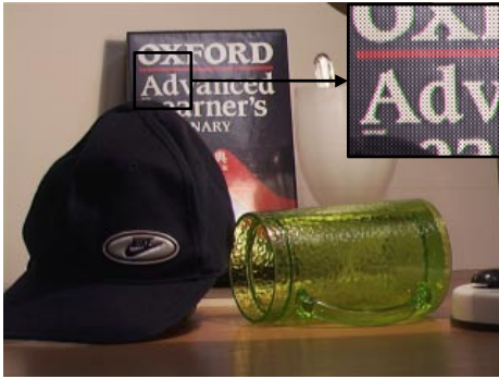
Figure 7: An SVE image with an exposure pattern that includes four discrete exposures.
