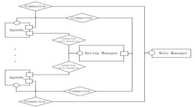
Figure 1: Architecture of distributed scheduling system
