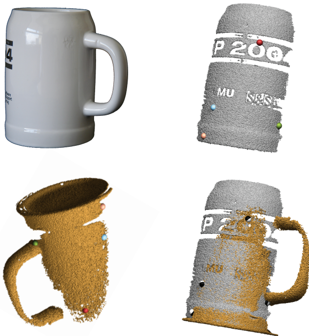
Figure 13: Alignment of slippable scans using 4PCS. The congruent 4-points bases are marked, colors indicating detected correspondences. With slippable bodies, 4PCS gives sub-optimal solution in the direction of slippage, like along the axis of the mug in this example. Here local descriptor based methods [Gelfand et al. 2005] degenerate to brute force search due to lack of distinctive features.
