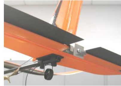
Figure 12. Razor blade fixed to the elevator to sever the perching line.
