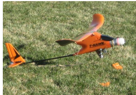
Figure 6. Sticky-Pad Plane prototype implemented with an AeroHobby "T-Hawk" R/C plane.
