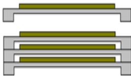
Figure 7. Sticky-Pad pucks stacked together.
