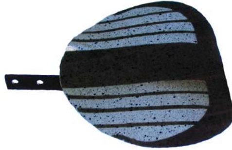
Figure 5. Speckled batten-reinforced membrane wing with wind tunnel attachment.
