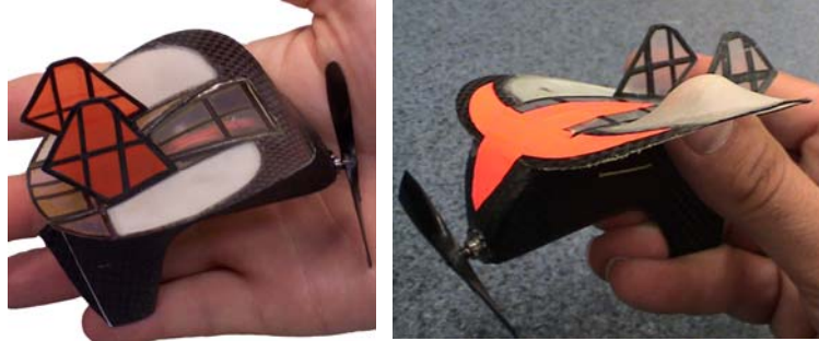
Figure 2. Perimeter-reinforced membrane wing design.
