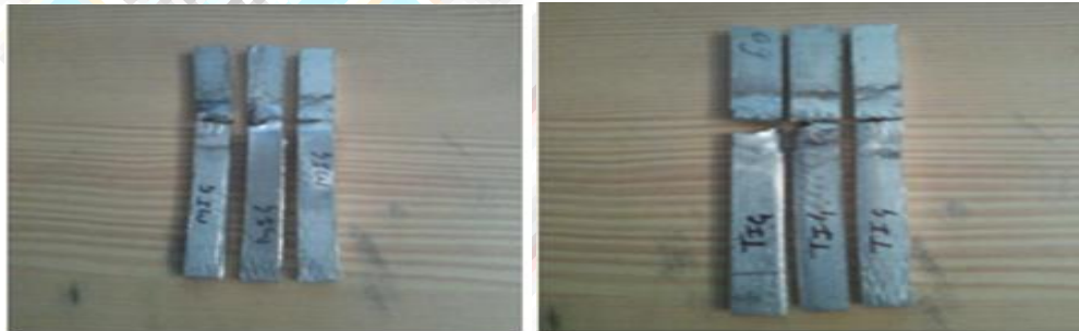
Fig. 1.10 MIG and TIG weld specimen after Izod test
