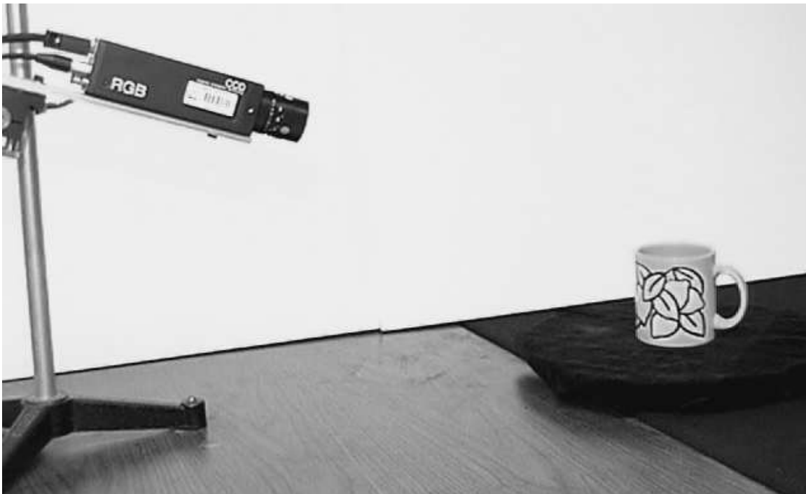
Figure 2: The objects were placed at the center of a motorized turntable. The turntable was rotated through 360 degrees. An image was acquired with a fixed camera at every 5 degrees of rotation.
