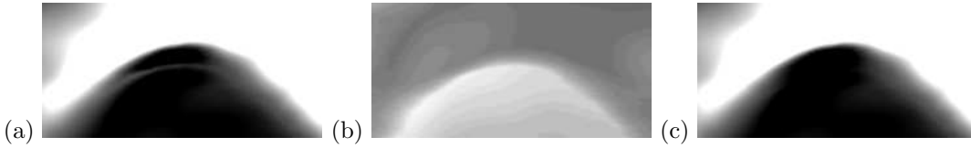
Figure 8: Artefact caused by large window and kernel changes over a short distance. (a) Region from DRS strain image at boundary between soft background and stiff inclusion phantom. Boundary appears twice because of excessive window and kernel overlap. (b) Window lengths (white=500 samples). (c) Window lengths have been clipped, thus eliminating the double-boundary artefact.
