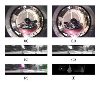
Fig. 4. (a) and (b) Images taken from stereo omnicameras in front of the vehicle. (c) and (d) Rectified perspective virtual views generated from the two omnicameras. The epipolar lines are along the rows of both the cameras. (e) Combined image. (f) Disparity map with pedestrians having large disparities [30].
