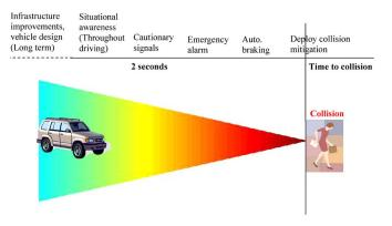
Fig. 1. Timeline of pedestrian protection measures (based on the study in [44]). The reaction time for a given distance decreases with vehicle speed.
