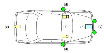
Fig. 3. Sensor configurations for detecting pedestrians and other objects. (a) Wide baseline stereo for distant objects. (b) RADAR for distance measurement in narrow FOV. (c) Narrow baseline wide FOV (omni) stereo pair for near objects. (d) Omnicameras to monitor blind spots. (e) Monocular reverse camera.
