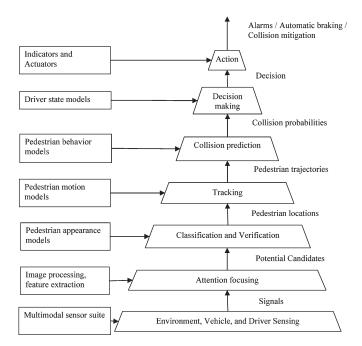
Fig. 2. Vehicle and infrastructure-based pedestrian detection. Data flow diagram showing distillation of information from raw signals up to appropriate action.
