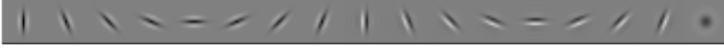
Fig. 5. Filters for creating textons. We use 8 oriented even- and odd-symmetric Gaussian derivative filters and a center-surround (difference of Gaussians) filter.
