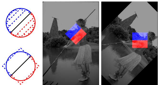
Fig. 22. Efficient computation of the oriented gradient of histograms. Left: The two half-discs of interest can be approximated arbitrarily well by a series of rectangular boxes. We found a single box of equal area to the half-disc to be a sufficient approximation. Middle: Replacing the circular disc of Figure 4 with the approximation reduces the problem to computing the histograms within rectangular regions. Right: Instead of rotating the rectangles, rotate the image and use the integral image trick to compute the histograms efficiently. Rotate the final result to map it back to the original coordinate frame.
