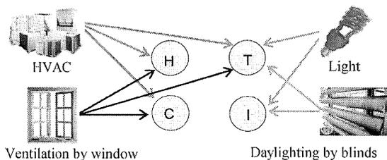
Fig. 1. Couplings of different devices on human comfort. T: temperature, H: humidity; L: illuminance; C: CO<sub>2</sub> concentration.
