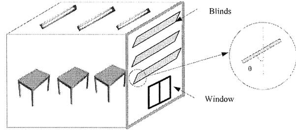
Fig. 2. A schematic of blinds, lights, and a window for natural ventilation.
