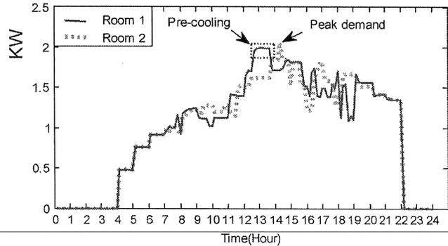
Fig. 4. Cooling power of the FAU and FCUs in two rooms.
