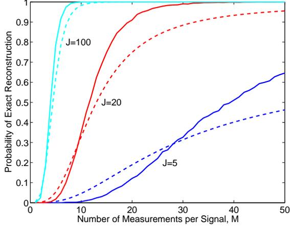
Fig. 1. Reconstruction using OSGA for JSM-2. Theoretical (dashed) versus experimental (solid) probability of error in recovering the support set  $\Omega$  in JSM-2 using OSGA for fixed  $N = 50$ ,  $K = 5$  and varying number of measurements  $M$  and number of signals  $J = 5$ ,  $J = 20$ , and  $J = 100$ . The theoretical formulation is presented in [8].
