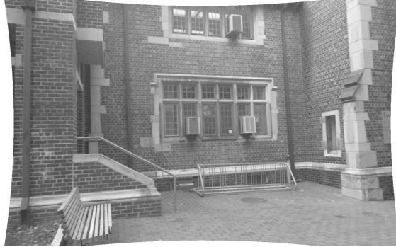
Figure 4: Correction of the Radial Distortion in a 853 \times 1280 image. The estimated distortion was 145.7 pixels at the image corner
