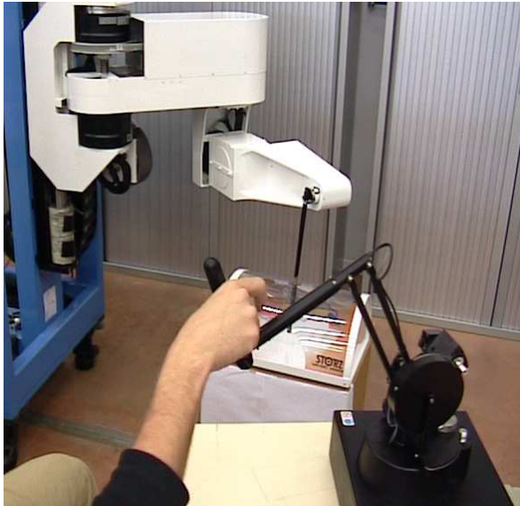
Figure 1: Experimental setup. D2M2 robot tele-controlled by the Phantom for robotic surgery. The medical instrument has 40 [cm] height.
