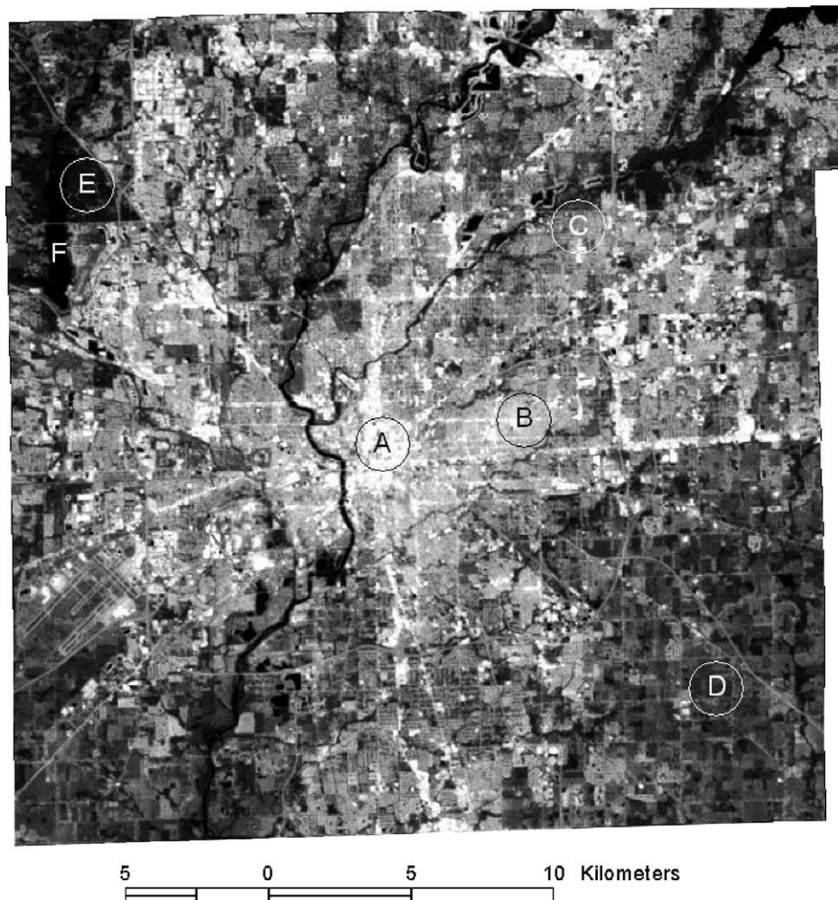
Fig. 2. Land surface temperature image derived from a Landsat 7 ETM+ thermal infrared band (land surface temperature ranges from 290 to 320 K, with lowest values in black and highest values in white): (A) commercial areas; (B) high-intensity residential areas; (C) medium-intensity residential areas; (D) agricultural lands; (E) forested lands; (F) water.
