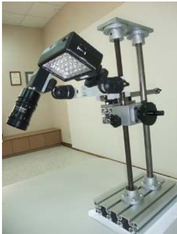
Figure 9. Prototype of scraping guide ways inspection device
