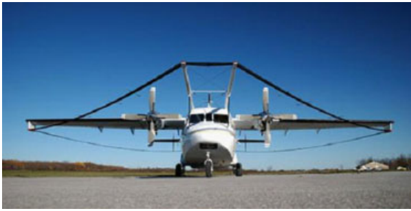
Figure 4. The Fugro airborne GEOTEM time-domain FWEM system
