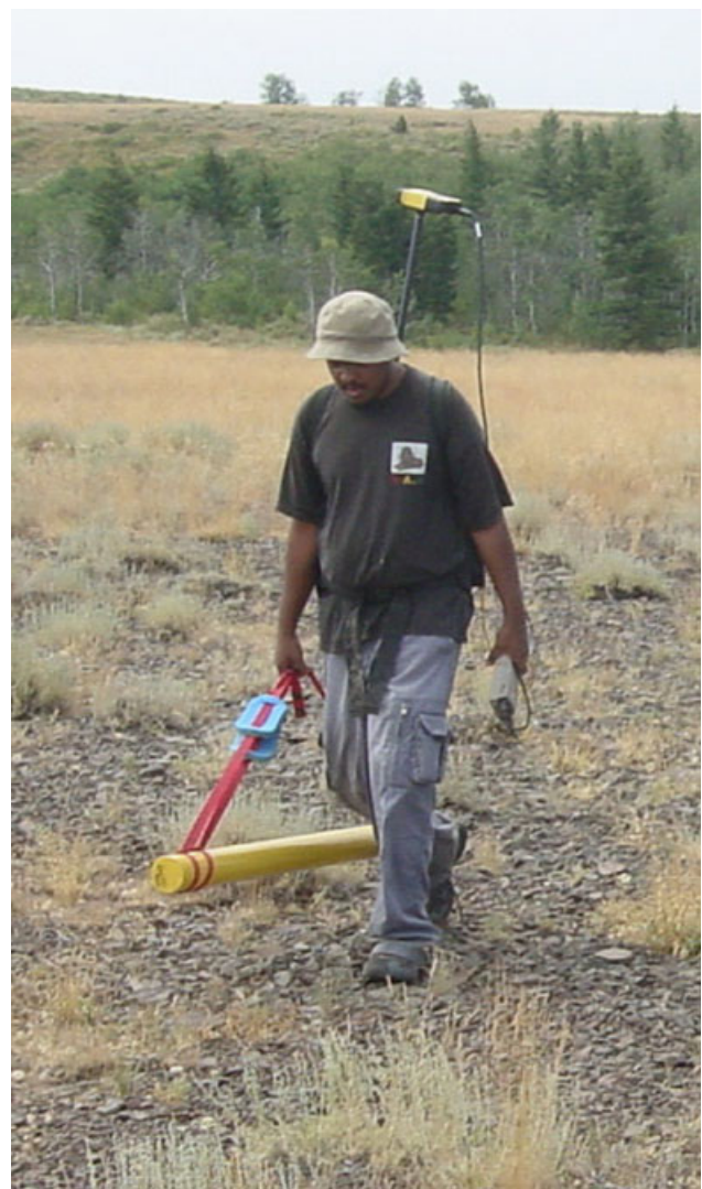
Figure 10. Field mapping ground conductivity using a Dualem EMI sensor at the USDA-Reynolds Creek experimental watershed in Idaho
