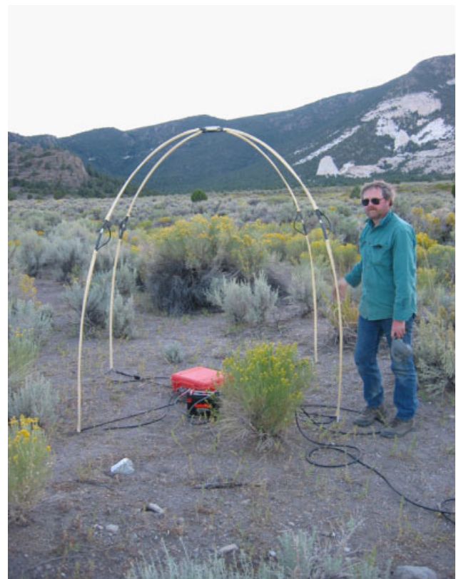
Figure 9. The StrataGem® AMT system (photograph courtesy of Geometrics, Inc.)
