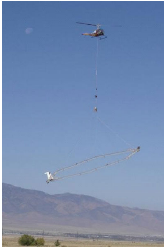
Figure 5. The SkyTEM HTEM system
