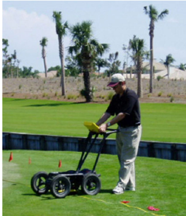
Figure 12. Noggin smart cart GPR (courtesy of Sensors and Software Inc.)
