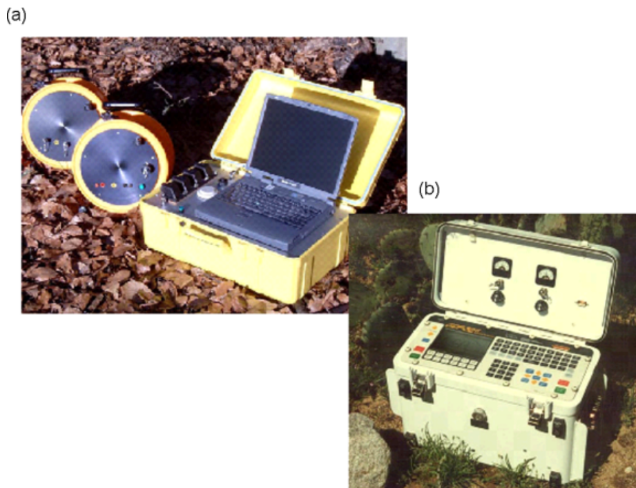
Figure 16. Examples of frequency domain SIP instruments: (a) SIP Fuchs II base unit and fiber optic cable reels; (b) Zonge GDP32 receiver
